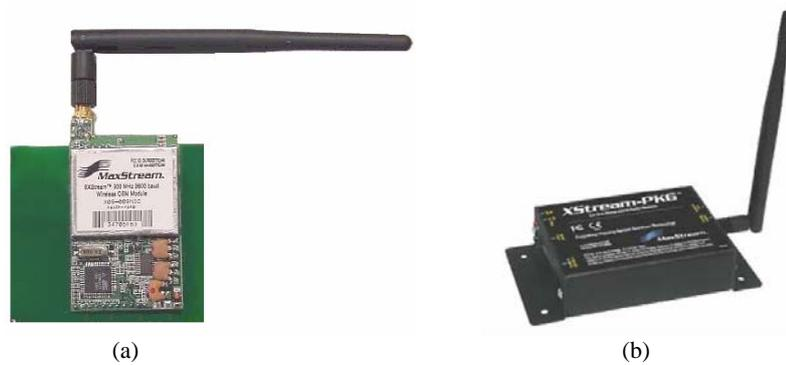
Figure 4. RF radio modem being considered for the project, a) For a PDS PCB and, b) For ground station.
