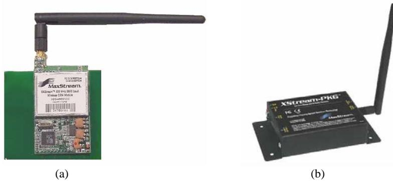
Figure 4. RF radio modem being considered for the project, a) For a PDS PCB and, b) For ground station.
